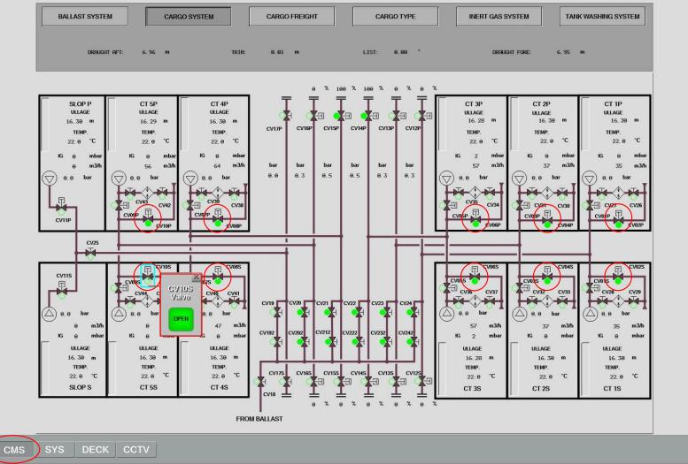
Open valves on drop lines for all other cargo tanks, except Slop Tanks.
