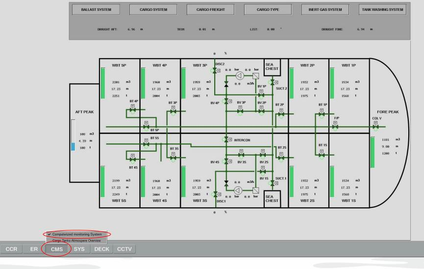
For open valves on drop line of cargo tanks # 3 P/S, you need to open valves on dropline in cargo tanks # 3 P/S. We are going to start loading into these tanks. Go back to the "CMS - Computerized Monitoring System - Cargo System" and open valves **CV06P** and **CV06S**.
