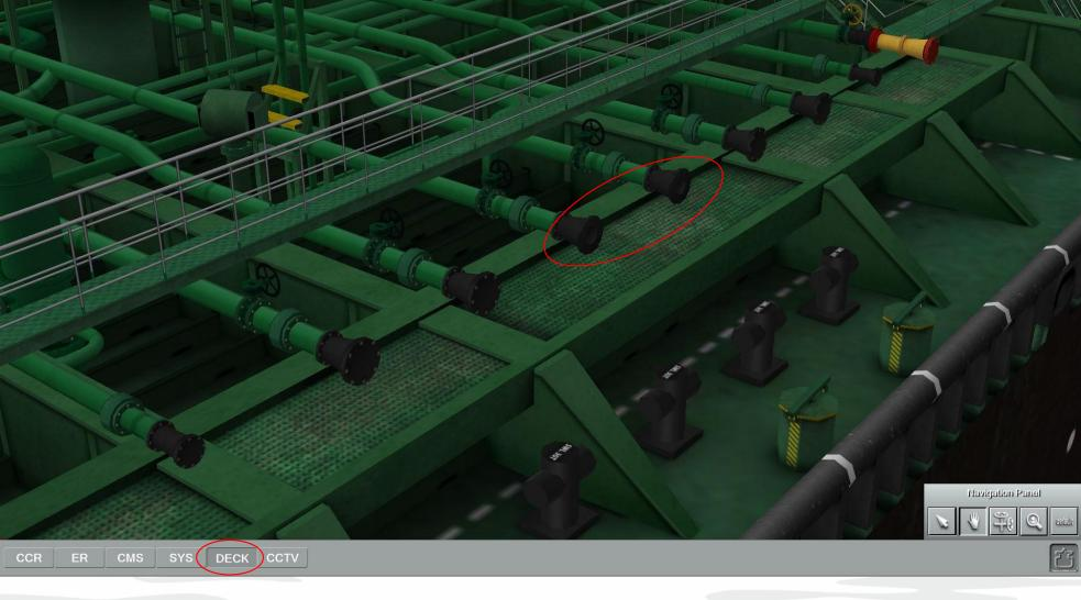
Check the condition of manifolds #3 and #4 portside – are the blanks off
