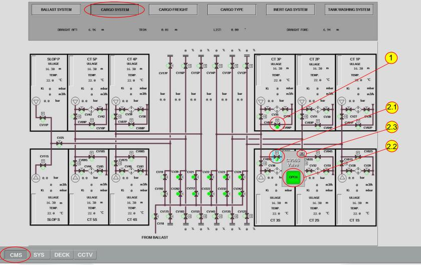
Open valves CV06P and CV06S. System is prepared. You need to inform shore terminal staff that we are ready for loading
